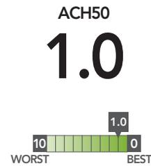
These results reflect Air Changes per Hour of measured air flow<sup>2</sup>.
